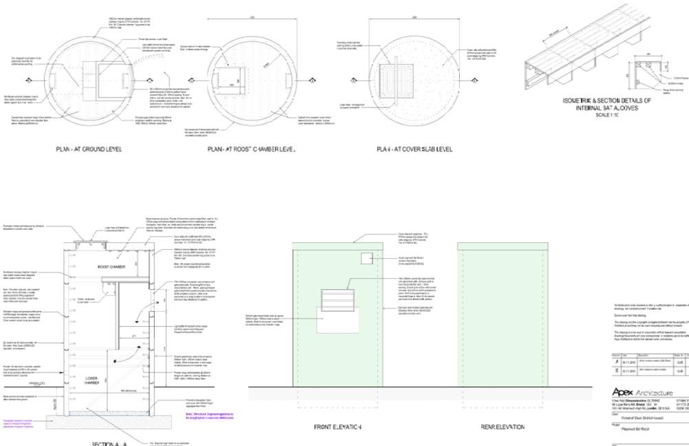
Our final design was based on pre-cast concrete sewer rings, with an internal baffle and upper chamber. An idea being that these could be prefabricated off site and transported and easily assembled on site.
